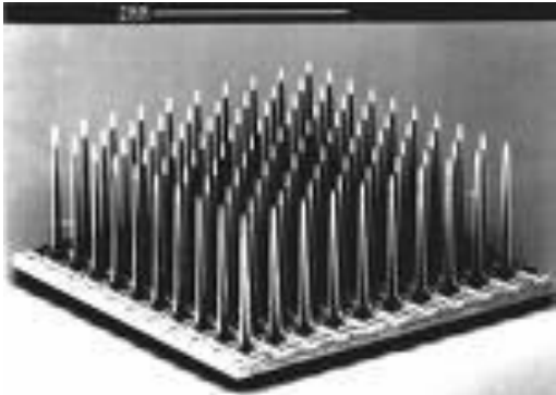
Utah Electrode Array 10 x 10 array of electrodes \frac{1}{4} " x \frac{1}{4} " in size
