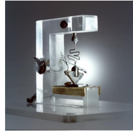
First Transistor, 1947 Bell Labs Discrete Transistor
