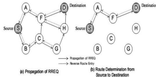
Figure 5 Propagation and route determination in AODV
